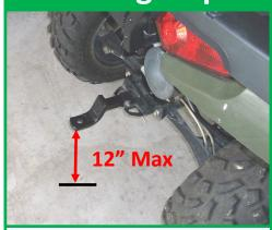
The device is intended for use with lawn tractors & ATVs that have a drop pin receptacle no higher than 1 foot.
