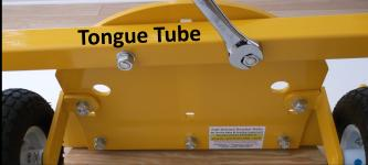
Remove tongue tube connection bolts with a 15/16", or 24mm, or adjustable wrench.
