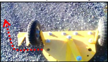
The Pull Behind Ratchet Rake is capable of angle grading crushed stone up to 1 1/4" in diameter. When the tongue tube is angled at 22 degrees, gravel is channeled through the rake and dispersed on the trailing side. Each individual tapered tine scrapes the driveways surface and causes a drag effect which enables the device to remain centered behind the tow vehicle. Loose gravel can be blended in to form the crowned profile with the rake set at 0 degrees.
