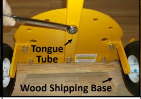
Reposition and secure the tongue tube on to the curved plate.
