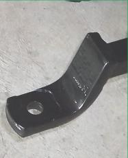
A standard ball mount (without the ball) can be used on machines that have a hitch receptacle.
