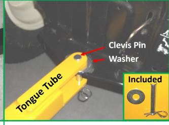
The tongue tube is connected to the machine's receptacle using the clevis pin. The washer is positioned under the tongue to reduce wear on the surface below.
